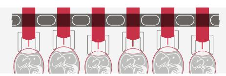
Special air tubes between the injectors inflate, locking the injectors in the ideal position. The injector head then makes a second fixed, downward movement, causing the injector's outer needles to pierce the shell collectively and precisely.
