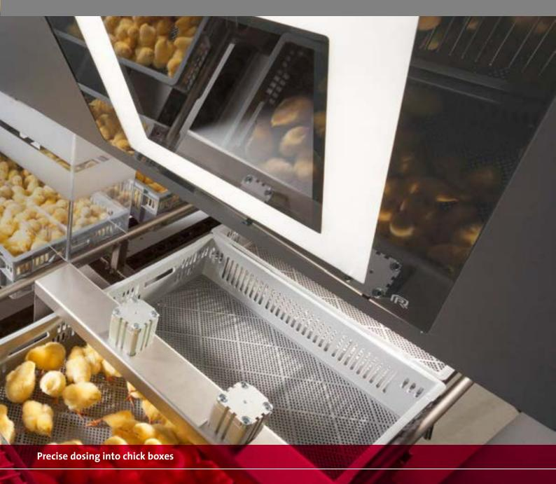
SmartCount™ uses Vision not only to count individual chicks, but also for pattern recognition, to deliver precise dosing of the day old chicks into chick boxes. The system's intelligent software adjusts conveyor speed based on numbers of chicks, to maintain accurate dosing in any conditions.
