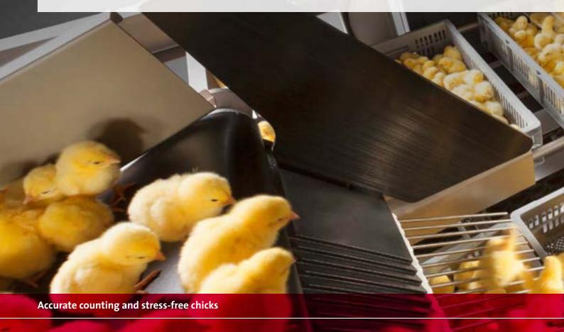
Unlike conventional chick counters, SmartCount™ does not require unnatural acceleration to separate the chicks. The system analyses sequential images of multiple birds.
